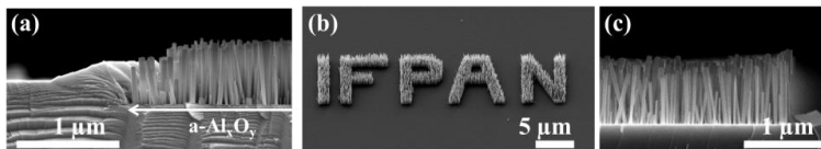
Fig. 1. SEM micrographs (a) of GaN NWs and the compact layer on the GaN/sapphire substrate with a- \text{Al}_x\text{O}_y stripe [3] and (b, c) of GaN NWs grown selectively on \text{SiN}_x/\text{Si} substrate with a- \text{Al}_x\text{O}_y nucleation pattern [4].
